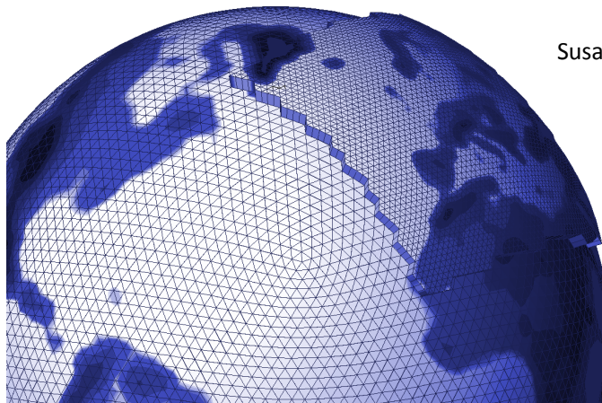
ICON grid with grid refinement over Europe. Figure by F. Prill (DWD)
